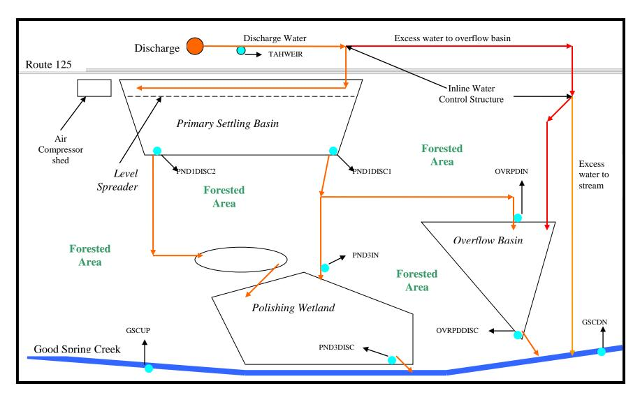
Tracy Airhole Discharge Treatment System Diagram and Sampling Locations
