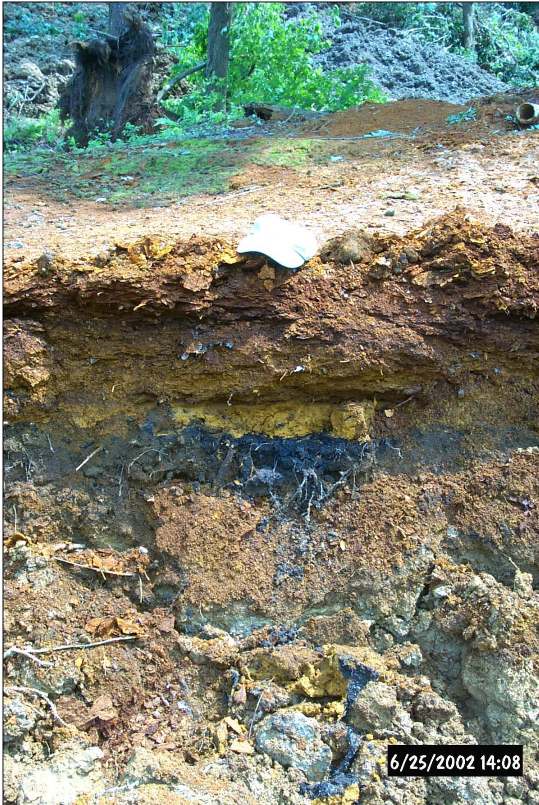
View of the soil profile during excavation of the passive treatment system. The top 1-2 feet was a thick “bed” of iron precipitates that had accumulated over the years from the abandoned mine discharge.
