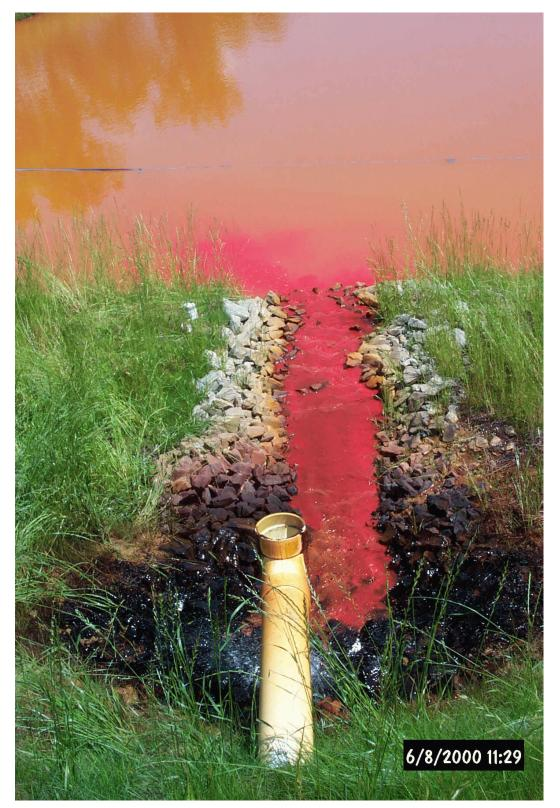
Beginning of dye test of Settling Pond #1 examining water distribution patterns.
