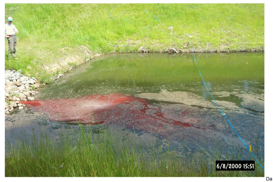
rcy Peart, Stream Restoration, Inc., looking over dye quickly moving through the HFLB.
