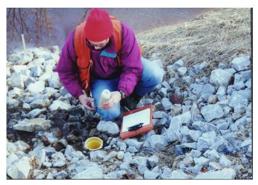
Tim Danehy, EPI, BioMost, Inc., sampling water from effluent pipe of Vertical Flow Pond. (12/17/99)
