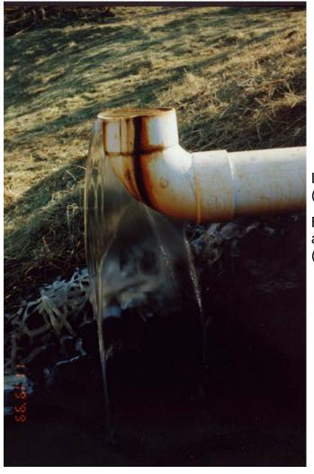
Left: Effluent from Anoxic Limestone Drain. (11/19/99)
