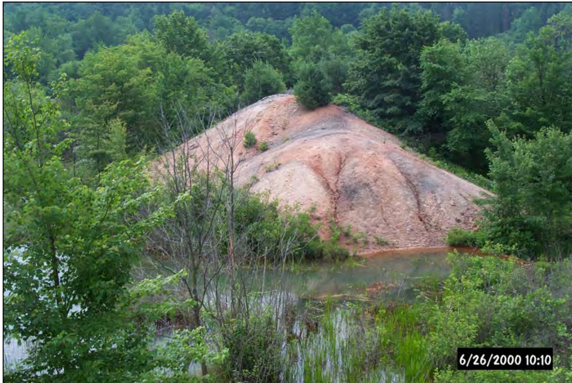
Views of the L-Shaped gob pile in Seaton Creek. Note the erosion gullies in the above photo. These gob piles contributed metals, acidity, and sediment to the stream. Also note the red color of the oxidized iron.
