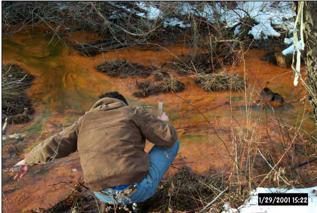
Tim Danehy, BioMost, Inc., carefully takes a water sample of the SR286 discharge. Several feet of iron had accumulated within the channel.
