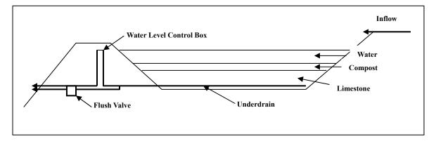
Figure 3. Diagram of Vertical Flow Pond.
