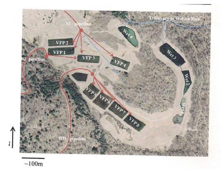
Figure AN1. The Anna S System treats the S1 and S2 discharges using VFP-1, -2, -3 and -4 plus Wetland Wet-4
