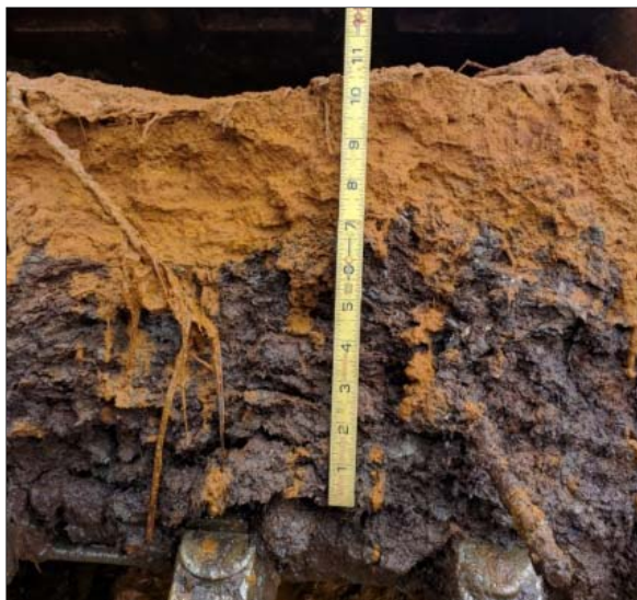
Left: VFR 2A and 2B had layered media which benefitted from the top layer being stirred to improve permeability. Top Right: VFR 2A after being stirred. Bottom Right: VFR 1 media was very compacted, shallow and had no observable limestone.
