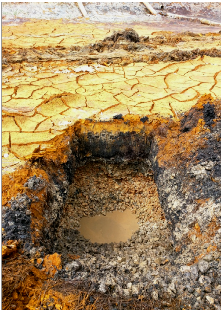
Left: VFR 2A and 2B had layered media which benefitted from the top layer being stirred to improve permeability. Top Right: VFR 2A after being stirred. Bottom Right: VFR 1 media was very compacted, shallow and had no observable limestone.
